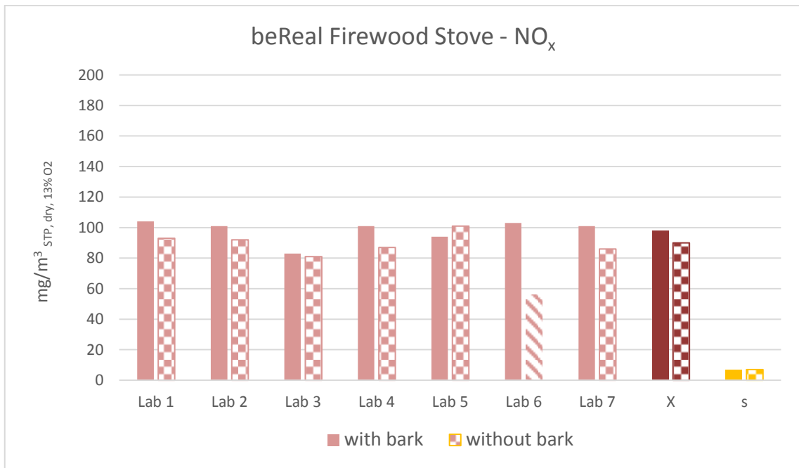
Figure 22 – Comparison of the beReal method for NO x using firewood with and without bark.
