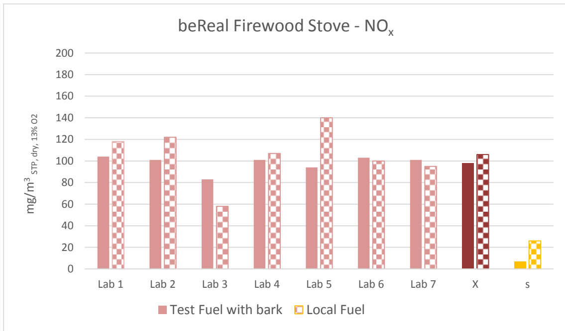
Figure 27 – Comparison of the beReal method for NO x using test fuel and local fuel.
