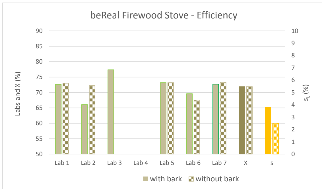
Figure 24 – Comparison of the beReal method for efficiency using firewood with and without bark.
