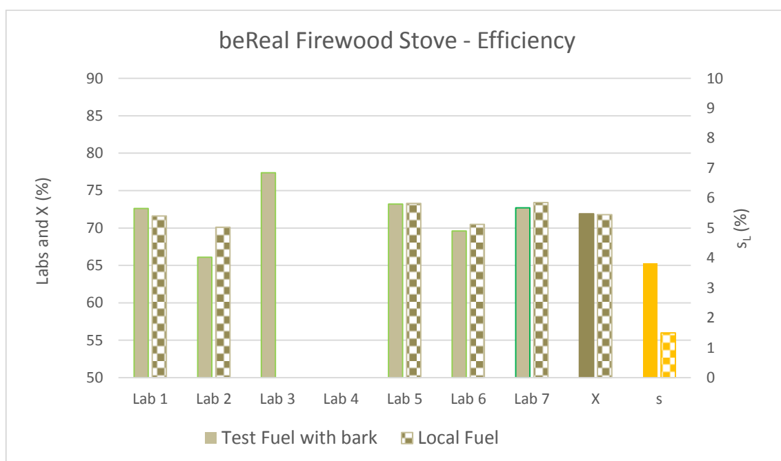
Figure 29 – Comparison of the beReal method for efficiency using test fuel and local fuel.
