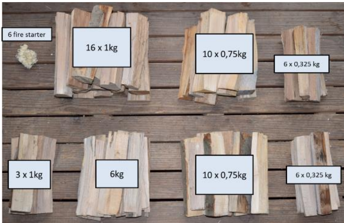
Figure 2 – The content of the “beReal fuel box” for wood stoves. The wood logs were prepared by the beReal project partner HFR.
