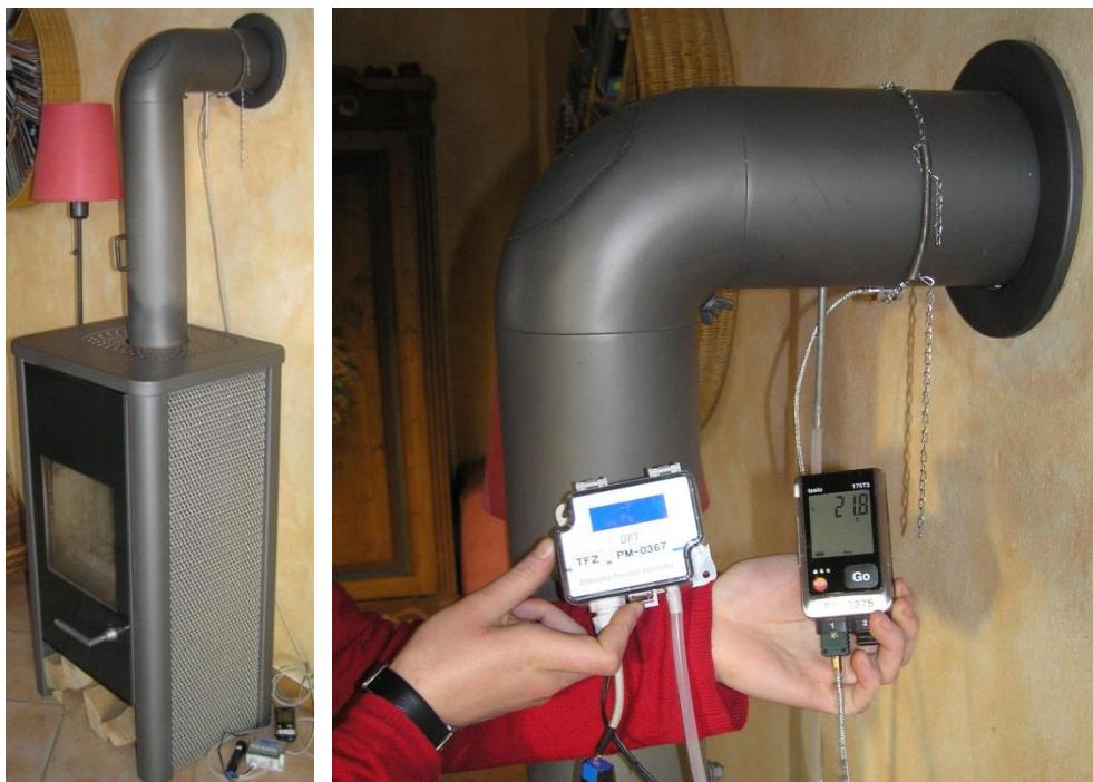
Figure 1: Chimney stove equipped with data logger for flue gas temperature and chimney draught measurement. Source: TFZ
